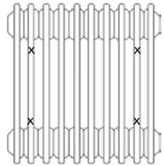
Universal Wall Brackets should be logically positioned to prevent Steel Multi Column radiators from falling away from the wall. If more than 4 brackets have been supplied these should be spaced evenly.
