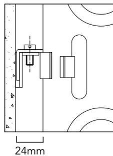
Fig 4 - Welded Feet
